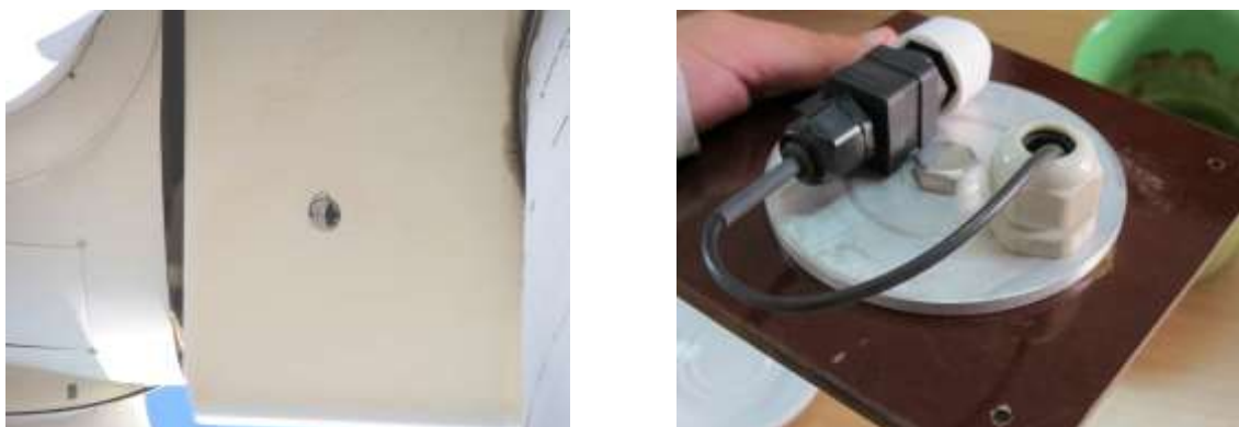
Figure 6. Installation of a bat detector system at VESTAS V47/660 kW wind turbine at CRES demonstration wind farm
